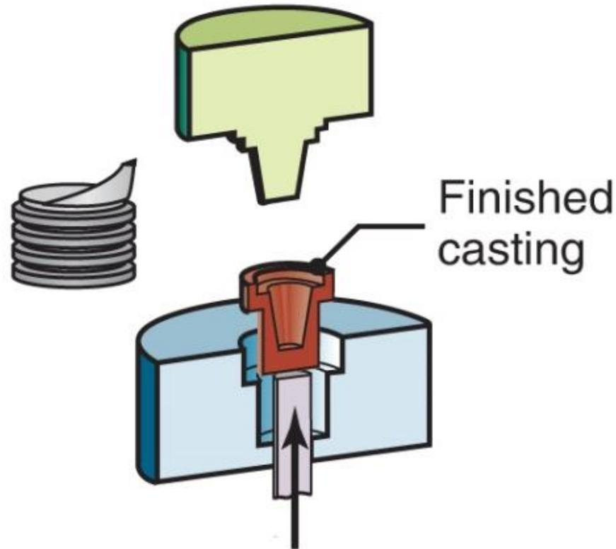
4. Eject squeeze casting,
